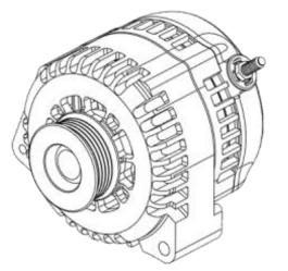
It is important that you increase the size of the battery charge wire to properly handle the higher amperage of your new alternator. In most situations the original charge cable can either be removed or can be left in place with an upgraded larger cable supplementing the stock charge cable. The larger supplemental charge wire can be fused within 12" of the battery terminal if desired for safety. Many OEM vehicles do not have any fusing in the OEM alternator charge cable.
