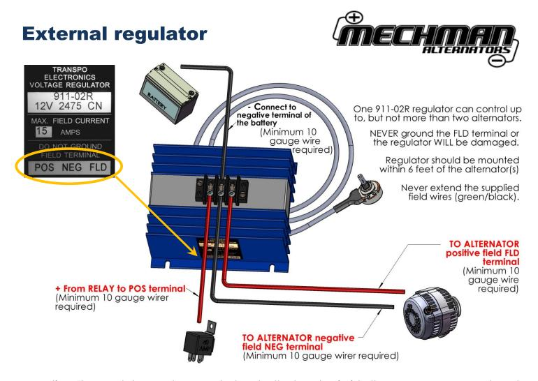
Mounting: The regulator can be mounted under the hood or inside the passenger compartment.
