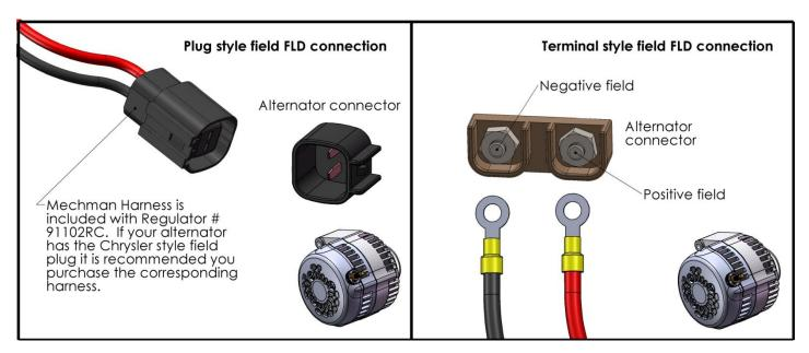
Regulator field connections at the alternator can be in the form of a plug, terminal(s), or wires.
